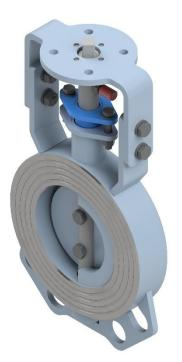
**CFM11** bidirectional butterfly damper valves with controlled leakage are suitable for max. 600°C working temperature and low pressure. They are used extensively for gas isolation or control application.
