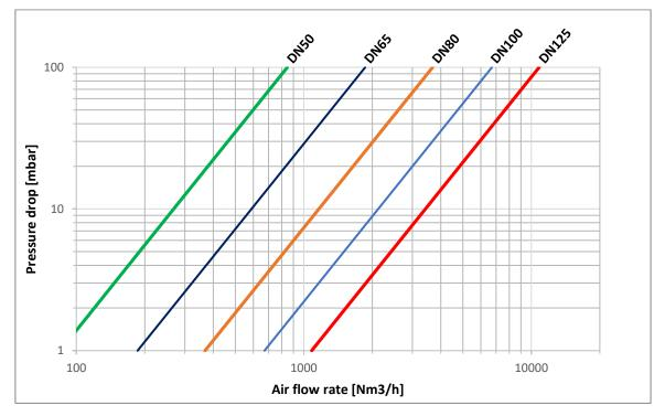
The pressure drop across the valve can be calculated with the following formula:
