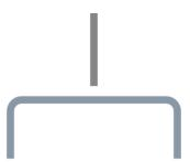
No contact between disc and valve body. Relative tightness class I FCI 70-2. Suitable when no specific tightness with closed disc is required.
