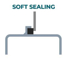
Soft gasket or braided seat between disc and valve body. It is designed to cater an improved tightness class requirement. Relative tightness class II FCI 70-2 (< 0,5% Kvs).
