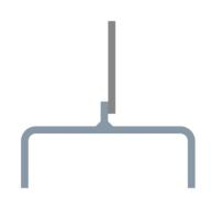
Metal seat with rigid rim between body and disc. This sealing option is widely used where a better shut off capability is required. It admits a percentage of leakage. Relative tightness class I FCI 70-2
